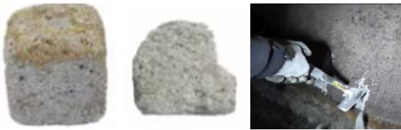
Fig. 6 & 7: OPC mortar containing fly ash, silica fume and silica sand after 1 year in an incubation chamber simulating the biogenic corrosion – the picture on the left being the cube at the start of the test and the one in the middle at 1 year later (3).
